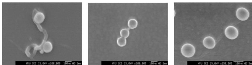
FIGURE 3 Scanning Electron Microscope (SEM) images of 190 nm of PS nanospheres chemically attached on the SWNTs.
